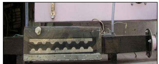
Figure 2. Systematic Arrangement of Ribs in duct.
